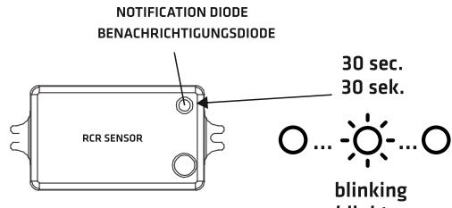
After turning ON the power, Indicator diode will blink for 30 seconds.
